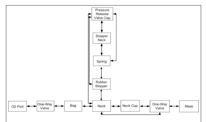
**Figure 3.** Block Diagram describing the interaction of the components of our bag valve mask design. Components interact with each other mechanically: an arrow could indicate that a component rests on another component, air travels through one component to the next, or that a component exerts a force on another component.
