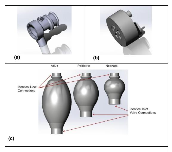
**Figure 5.** (a) Our neck design with a universal bag connection. (b) Our oxygen port design with a universal bag connection. (c) Our bag design with a universal connection for our neck and oxygen port.
