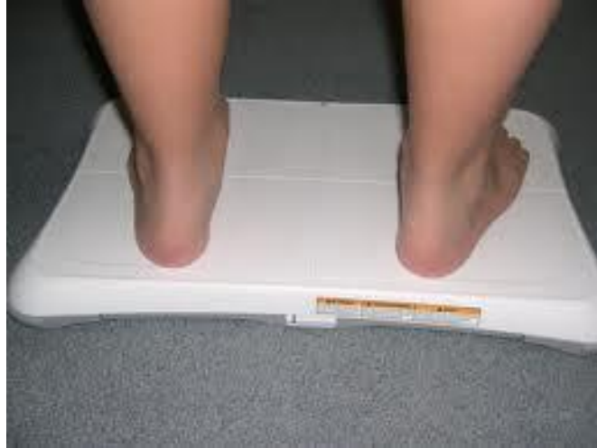
(fig a.) Picture shows a Wii balance Board. Transducers in each corner measure forces across the board and accurately calculate the weight distribution across the device. In our design it will communicate with a microprocessor via bluetooth to relay the distribution.
