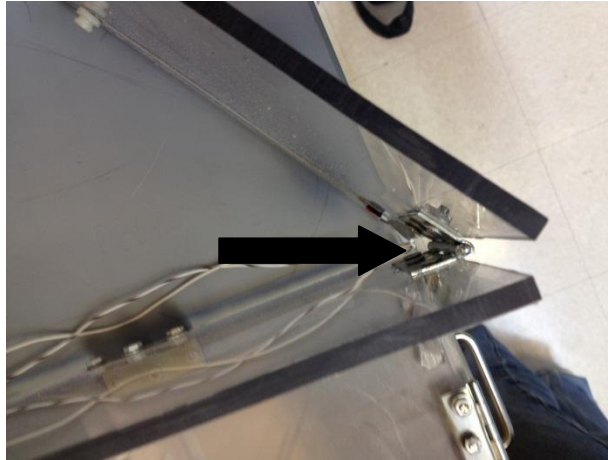
Figure 10: The arrow above points to the hinge connecting the top and bottom layers of the plate.
