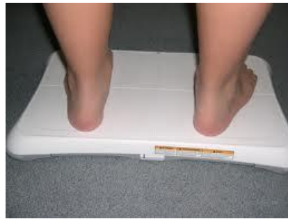
Figure 1: Picture shows a Wii balance Board. Transducers in each corner measure forces across the board and accurately calculate the weight distribution across the device. In our design it will communicate with a microprocessor via bluetooth to relay the distribution.
