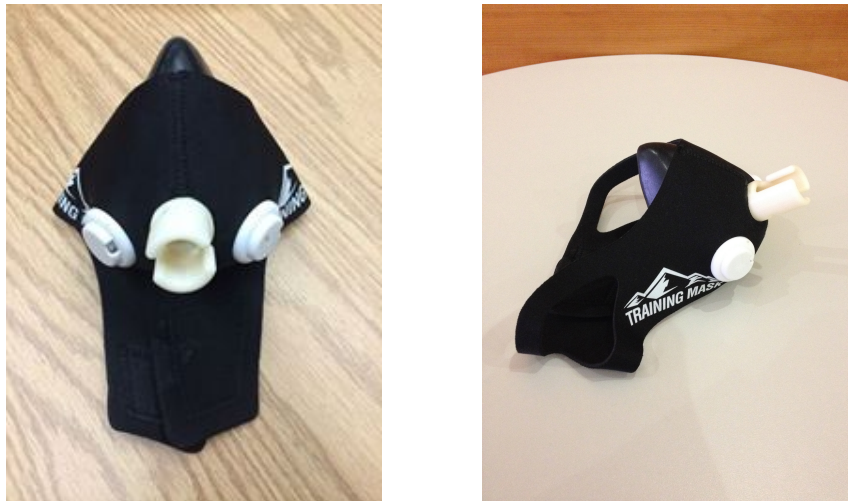
Figure 17: Modified Elevation Training Mask 2.0. Contains a silicon nasal/mouth shell, outer neoprene sleeve, dead space attachment at central port, and sensor attachment at lateral ports.
