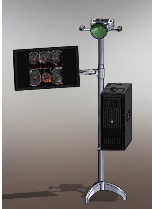
Figure 3: The Wii remotes require an IR lamp to increase accuracy. The entire setup, including the central computer and display unit, is shown. One Wii remote is placed on either side of the IR lamp at the top of the apparatus.
