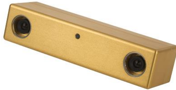
Figure 6: The Bumblebee2 contains two cameras and can accurately determine 3D location without the need for another optical input [7].
