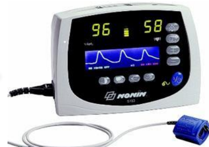
Figure 2. Nonin's Avant 9700 oximeter displays both graphical and numerical data. 8
