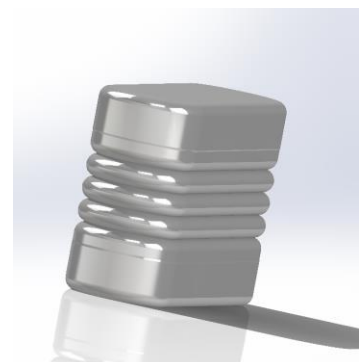
Figure 6: SolidWorks rendering of Inflatable Reinforced Distractor
