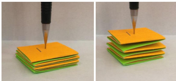
Figure 8: Accordion device in various degrees of inflation
