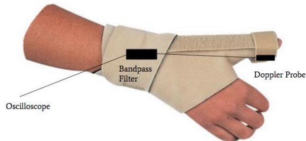
Figure 7. The probe will still be wrapped within the splint, but the signal will first be sent through a bandpass filter to further reduce any potential noise[9].
