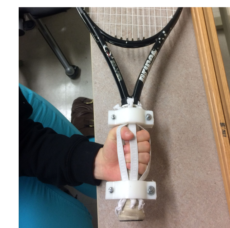
Figure 12: Close view of racket grip design in use
