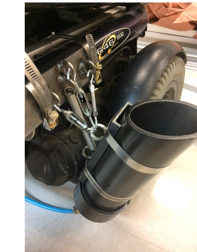
Figure 8: Launching tube attachment with tube
