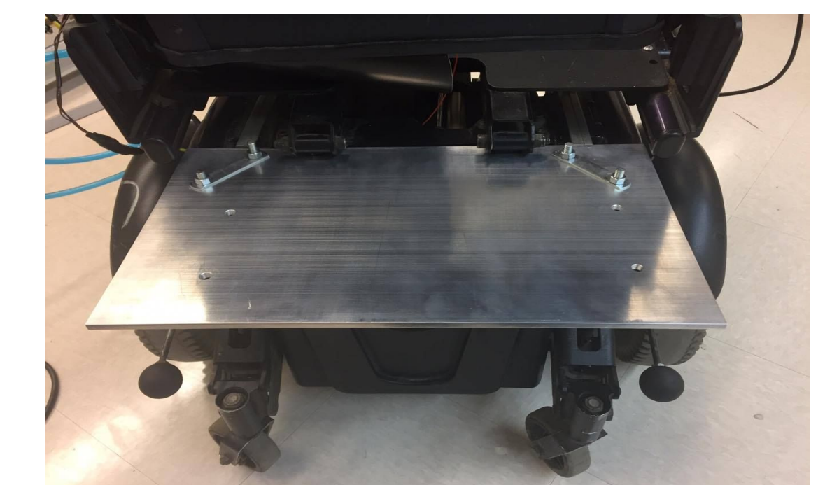
Figure 9: Tank attachment fixed to wheelchair bar
