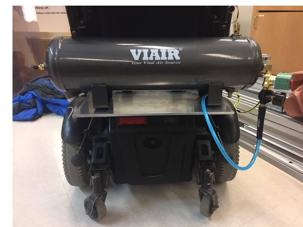
Figure 5: Launching system tank on back of wheelchair
