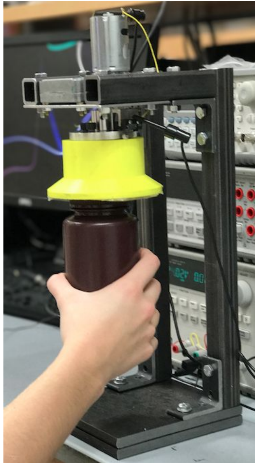
Figure 8: The final prototype in action. A user presses the container upwards into the cone, causing a snap-action switch to activate the motor. The motor revolves the high friction cone (clockwise) until the cover is removed. The user relieves the pressure from the container stopping the motor.
