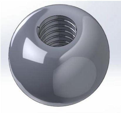
Figure 8: SolidWorks design of threaded recipient site
