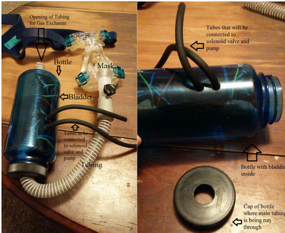
Figure 7 (left): This image shows our device prior to insertion of the circuitry. The bladder is visible inside of the bottle. Rubber bands around the bladder aid in diffusion once the pump is turned off.
