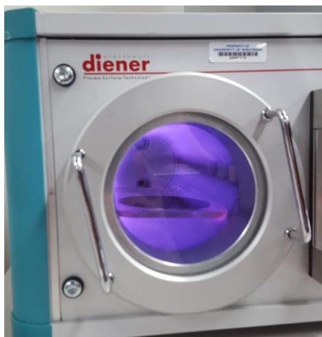
**Figure 12:** Picture of the plasma treatment of PDMS channels as well as glass slides.
