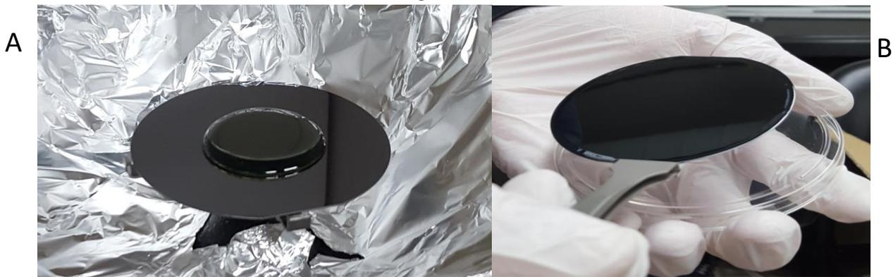
**Figure 9:** *A) Picture of the silicon wafer with approximately 3-4 mL of SU-8 50 placed on top. B) Picture of the silicon wafer and SU-8 50 layer post spinning to apply it evenly along the wafer.*
