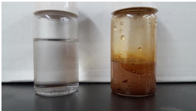
**Figure 17:** Picture of the two ferrofluid solutions created for testing. Ferrofluid mixed with ethanol (Left). Ferrofluid mixed with water (Right).
