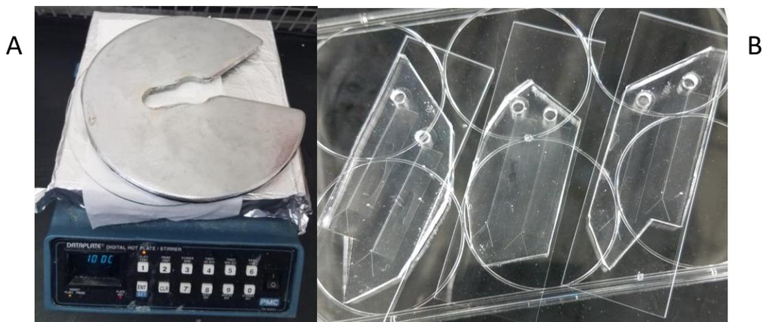
**Figure 13:** A) Picture of pressure being applied with a weight to permanently bond the PDMS channels to the glass slide after plasma treatment. B) Picture of 6 channels produced after permanent attachment via plasma treatment.
