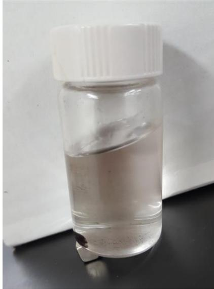
**Figure 18:** Picture of the ferrofluid/ethanol solution in a glass vile. Neodymium magnet placed underneath to draw ferrofluid particles out of solution. Shown to strongly congregate around the magnet.
