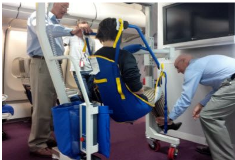
Figure 4: EagleLift. This design incorporates a hammock like design to lift the user into the chair in an easier manner.
