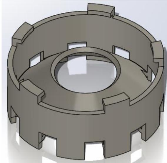
**Figure 8.** Final LED sample holder from last semester
