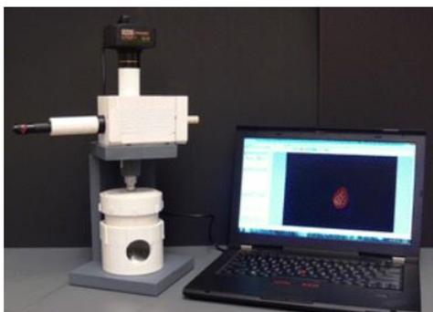
**Figure 6.** OPN-Scope Open Source Fluorescence Microscope System
