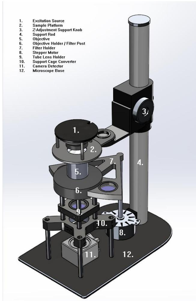
**Figure 7.** Overview of proposed microscope structure. A legend is included to identify all important components of the design.
