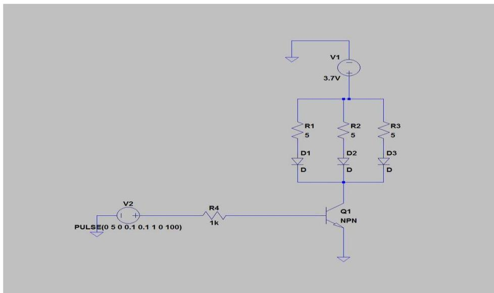
Figure 10. Schematic of circuit for excitation source.
