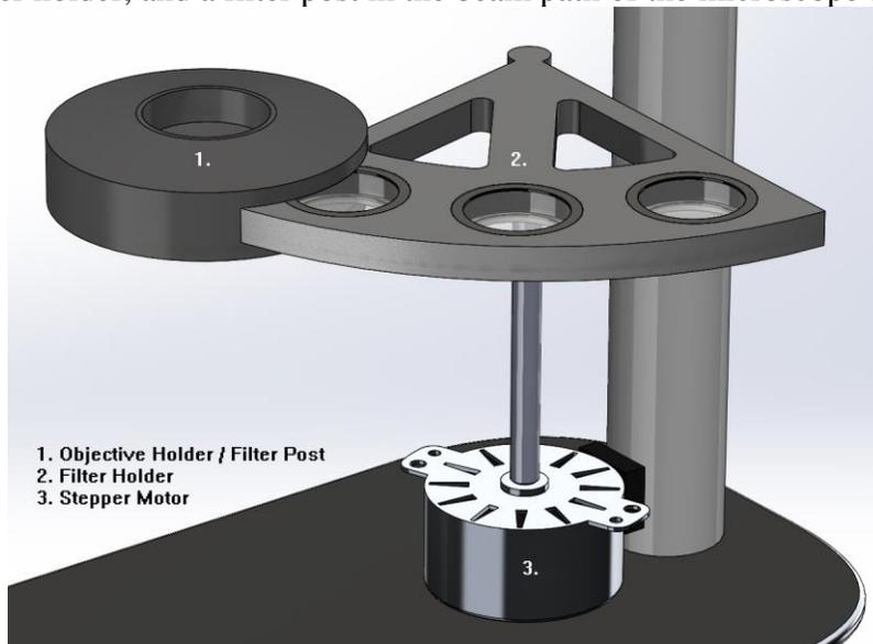
**Figure 9.** An exploded view of the filter swapping mechanism. This system shares the role of also supporting the objective (not shown). The stepper motor attached to the microscope base will provide the input to switch filters between images.
