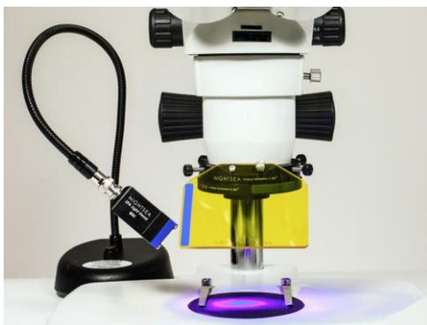
**Figure 5.** The NightSea Model SFA [9] consists of an excitation source and a filter that attaches to stereoscope.
