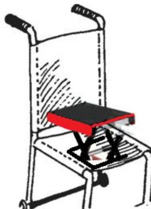
Figure 3: Scissor Lift preliminary design drawing
