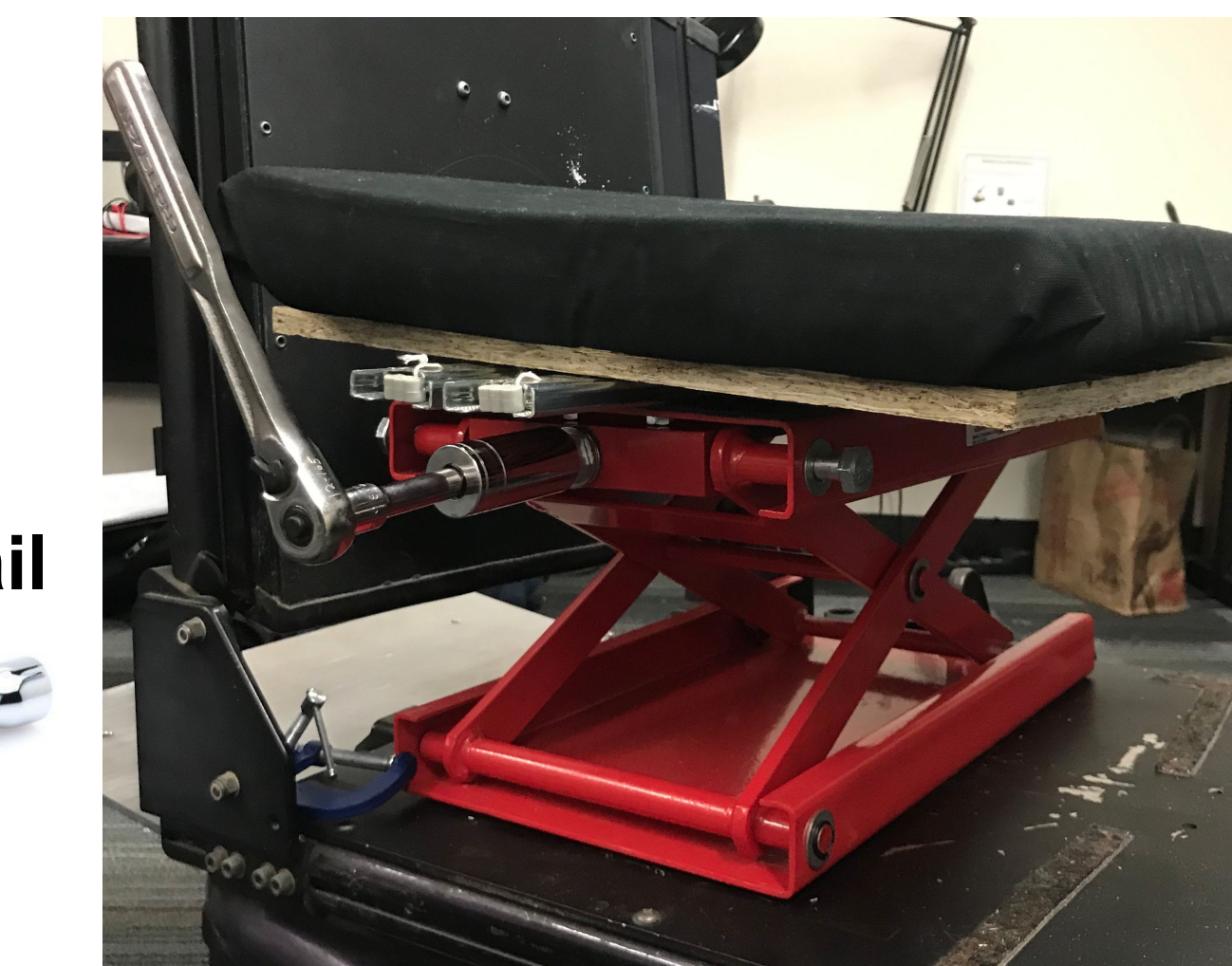
Figure 9: Finished design on wheelchair
