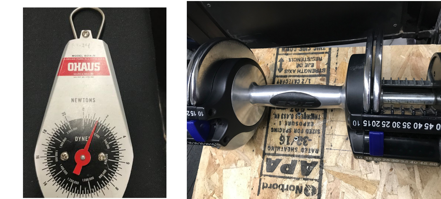
Figure 4: The first picture shows the Newton force meter used to measure the force required laterally. The second picture shows weight on the device.
