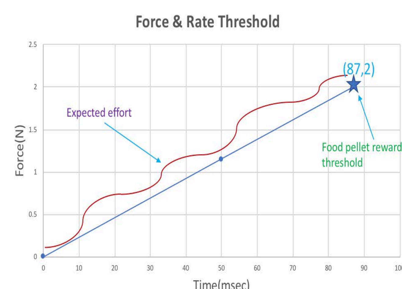
Figure 3: This graph depicts the idea that as long as the rat applies more force than the reference force over time (shown above by the blue line) the linear actuator will continue to pull on the rat's arm until the target force is reached.
