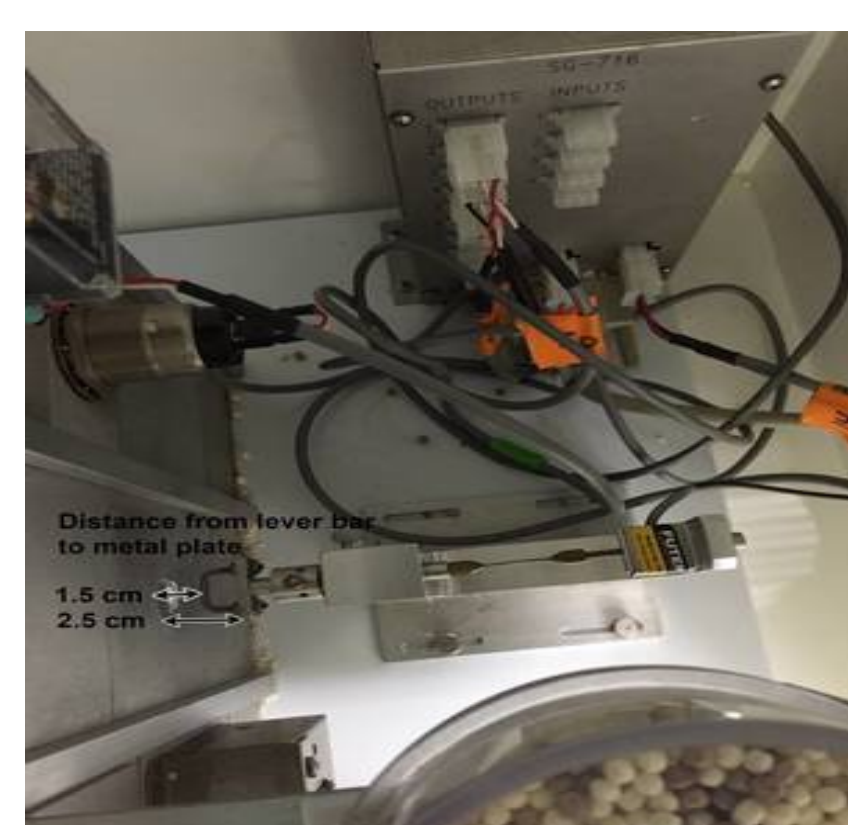
Figure 2: As shown in the picture above, the handlebar will be 2.5cm from the slot in the cage wall, distance from window to handlebar: 1.5cm
