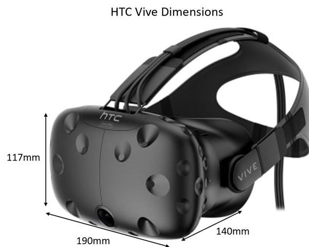
[Figure 4] A schematic of the HTC Vive's dimensions. The image was retrieved from [10].
