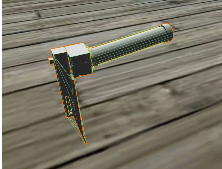
Figure 34: Unity uses a system of meshes to calculate collision physics, parsing the object into triangles, as pictured above. The described haptic software will calculate collisions based on evenly distributed points along the surface of the tool.
