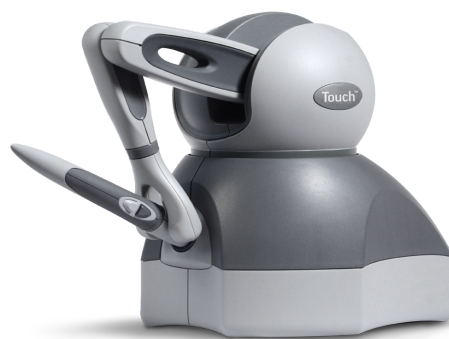
Figure 2: The image depicts a PHANToM Touch (3D Systems), comprised of a handheld stylus attached to a motor arm. The device interacts with an independent computer running Geomagic software via USB [28].
