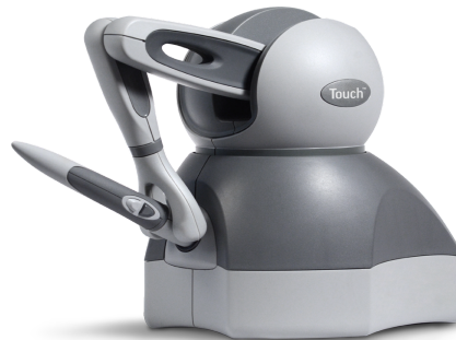
Figure 2: The image depicts a PHANToM Touch (3D Systems), comprised of a handheld stylus attached to a motor arm. The device interacts with an independent computer running Geomagic software via USB [26].
