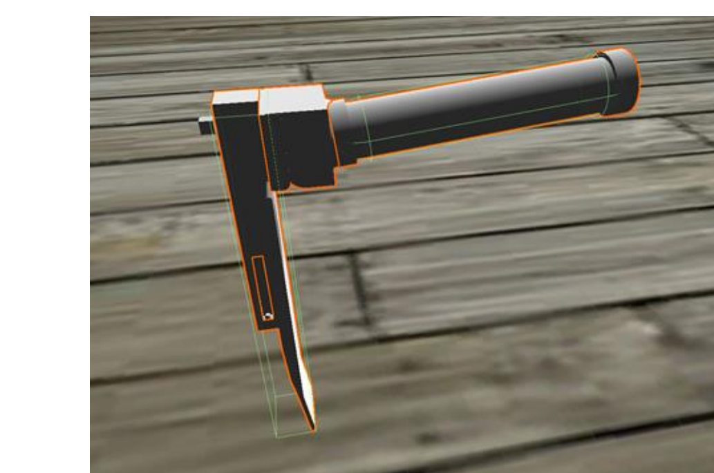
Figure 7: Points covering the surface of the laryngoscope will be used with a collider, producing linear forces and torque around a central axis
