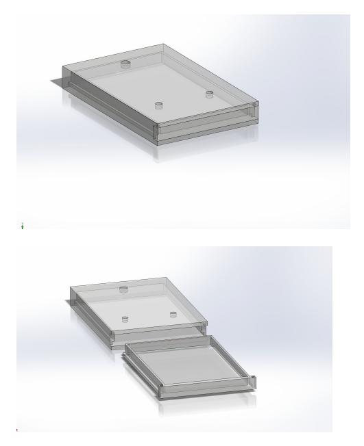
This design contains two parts. The first part is the main frame, and the second part is the platform. The material for the main frame will be PDMS, which is biocompatible, oxygen preamble, and highly transparent. Its size is 76mm x 50mm x 10mm. The size of the device
