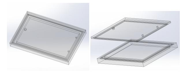
This design contains a lid and a base part with an overall dimension of 68mm\*44mm\*6mm. The base part has a 3mm deep camber inside the base and 0.75 mm deep continuous grooves on the sides. The lid part has 1mm continuous extrusions that can fit into the groove, sealing the chamber while leaving space for open it. Three pores are located at the lid: the larger one is for the input of the plant seed and two smaller ones are inlets for different bacteria. All the structures
