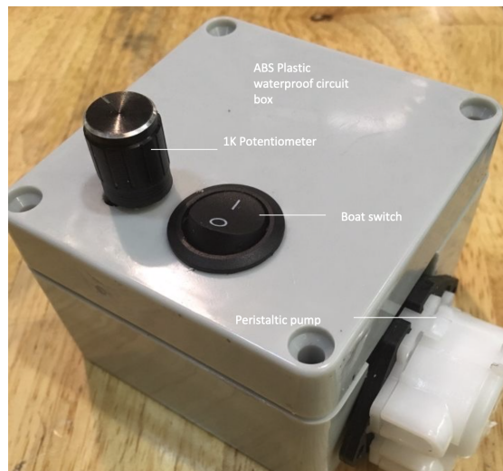
fig 1 Final circuit component, assembled in a circuit box
