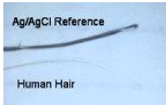
Figure 11: Electrodeposited Ag/AgCl reference electrode alongside a human hair.
