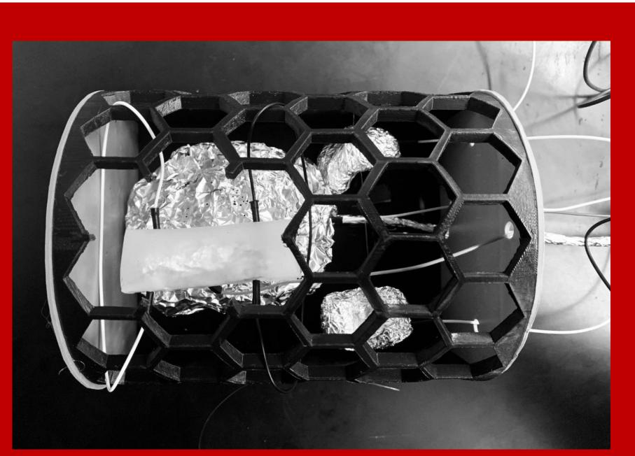
**Bladder Representation**  Aluminum base and ecoflex can be handled in a manner similar to palpation • Approximate size of a full bladder
