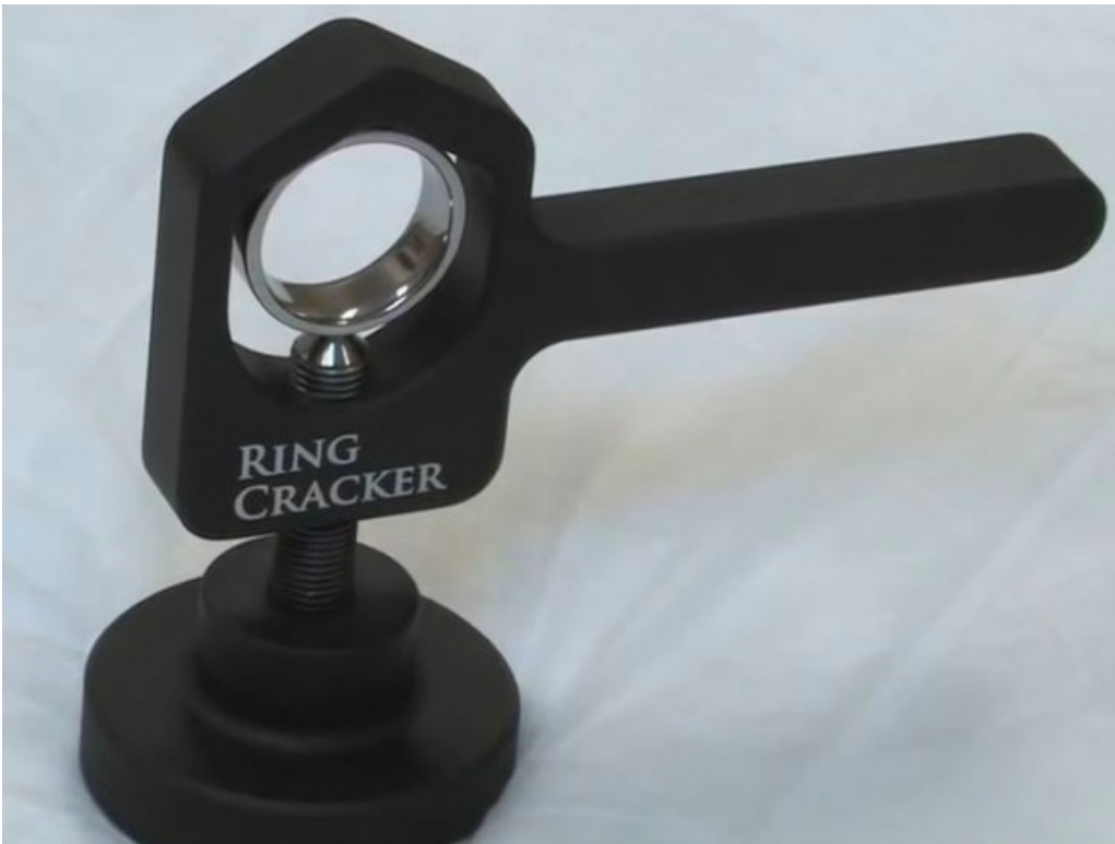
Fig 1. The Ring Cracker Device that is currently in the market. The pointed screw is turned by the black knob, tightening the Tungsten Carbide ring.
