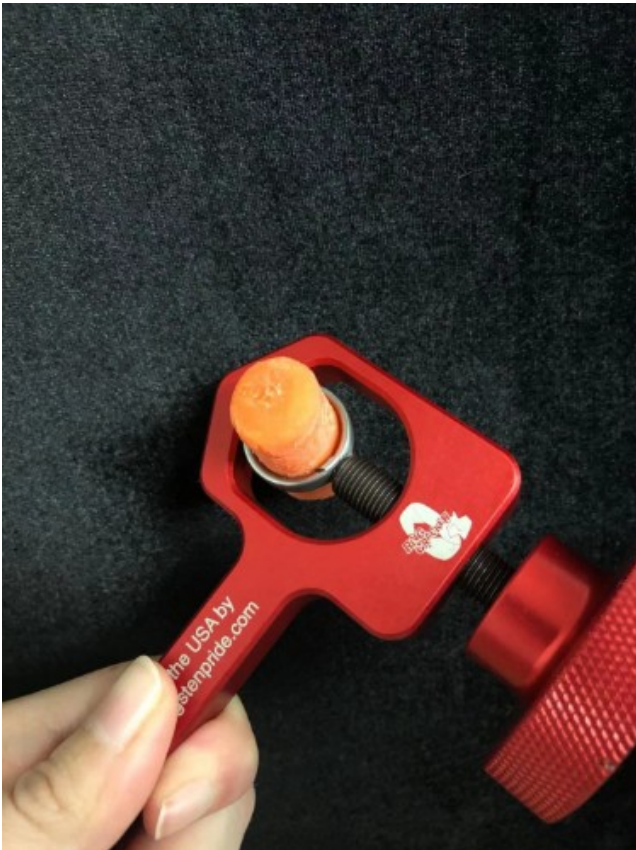
Figure 1. The carrot is used to mimic the finger with the ring cracker and tungsten carbide ring in.
