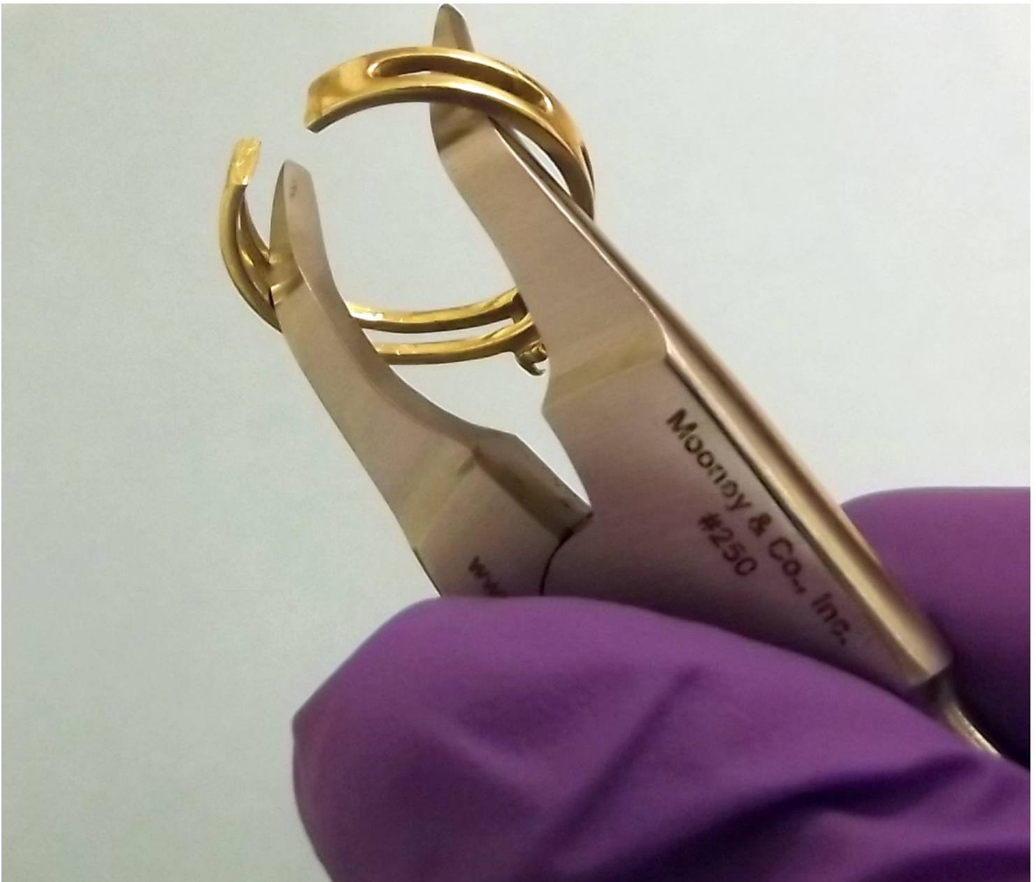
Figure 2. Once the initial cut of a constricting band has been made, the ring still may not be easily removed from the limb or finger. A ring spreader is designed to painlessly spread bands for removal without the need for an additional cut.
