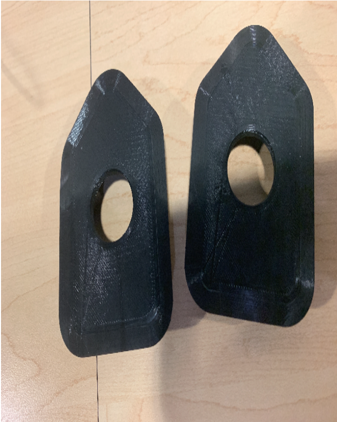
Figure 1. The new prototype of ring cracker protection system using black PLA
