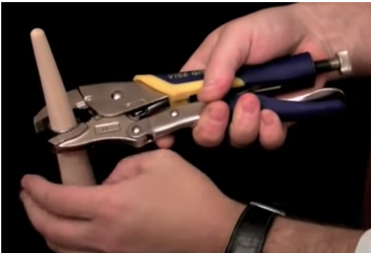
Figure 2. The process of using a cutter to cut the tungsten carbide ring
