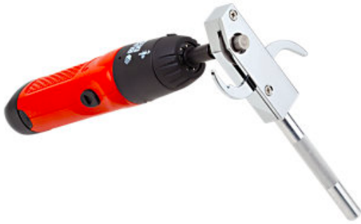
Fig 3. Electric ring cutter with battery powered drill
