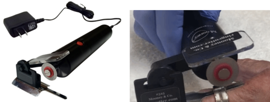
Figure 1. The components of the Gem Ring Cutter Emergency Ring Removal System (left), when the device is applied to the rings in real surgery (right).
