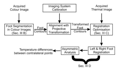
Fig. 3 Schematic flowchart of the proposed methodology for automatic detection of diabetic foot complications.
