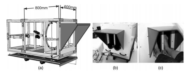
**Fig. 2** The experimental setup for foot scanning: (a) the schematic of the experimental setup with two cameras installed, which are the thermal camera (upper) and the RGB camera (lower). (b) The appearance of the experimental set and (c) positioning of patients' feet during measurement.
