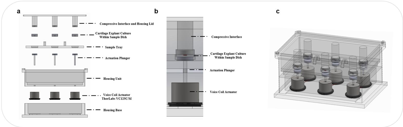
**Figure 4.** An overall depiction of our end-of-year analytical prototype. Exploded [a], unit [b], and trimetric [c] views are provided. Perspective [b] depicts active compression of the cartilage sample, with housing components left unlabeled to direct focus to active components within the bioreactor.
