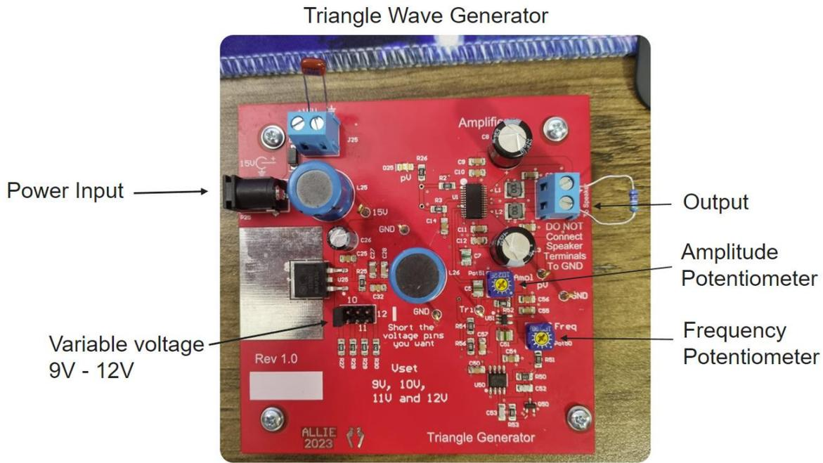
**Figure 10.** PCB board designed by Dr. Mark Allie.
