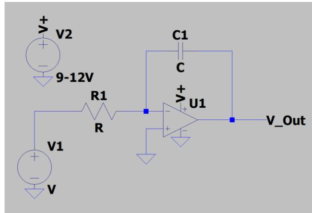
**Figure 8.** General circuit schematic to drive the voice coil.
