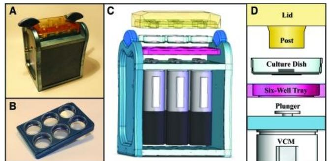
**Figure 3.** Prior work provides inspiration for the overall schematic build of a force-controlled cartilage bioreactor.
