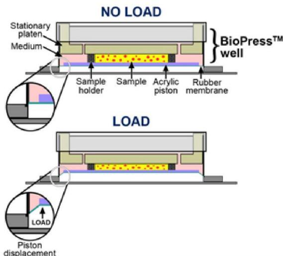
**Figure 7.** Flexcell's FX5000C compression system hydrostatic actuator in loaded and unloaded conditions [11]. Notice the membrane deflection in the circle on the left.
