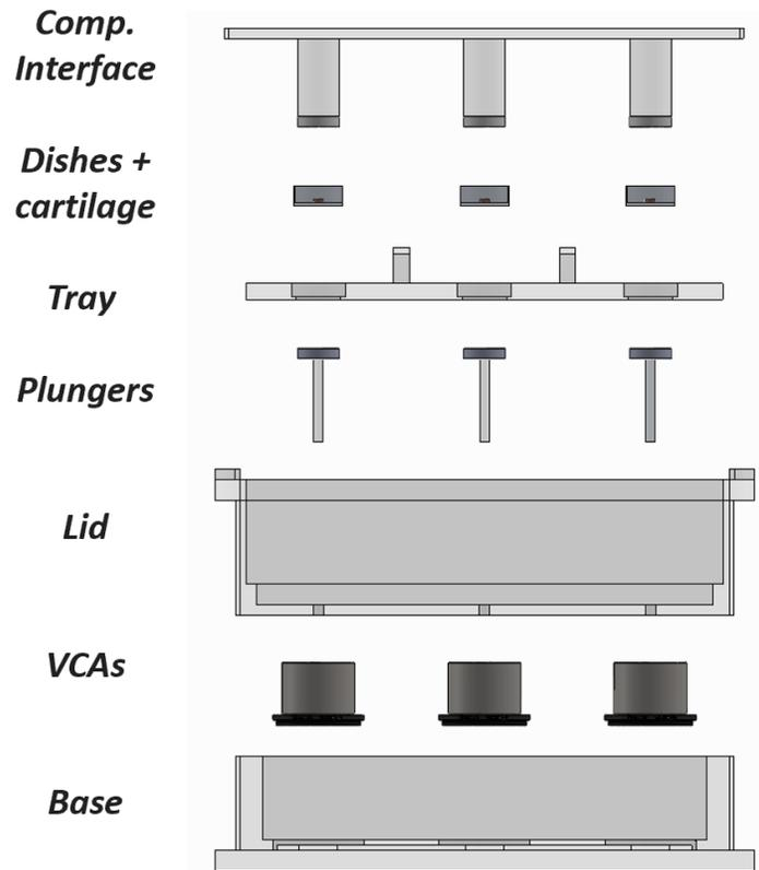
**Figure 12.** Exploded view of the bioreactor with its components labeled.
