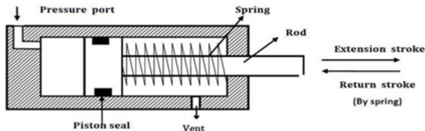
*Figure 6.* A general schematic illustrating how a spring-return actuator operates [9].
