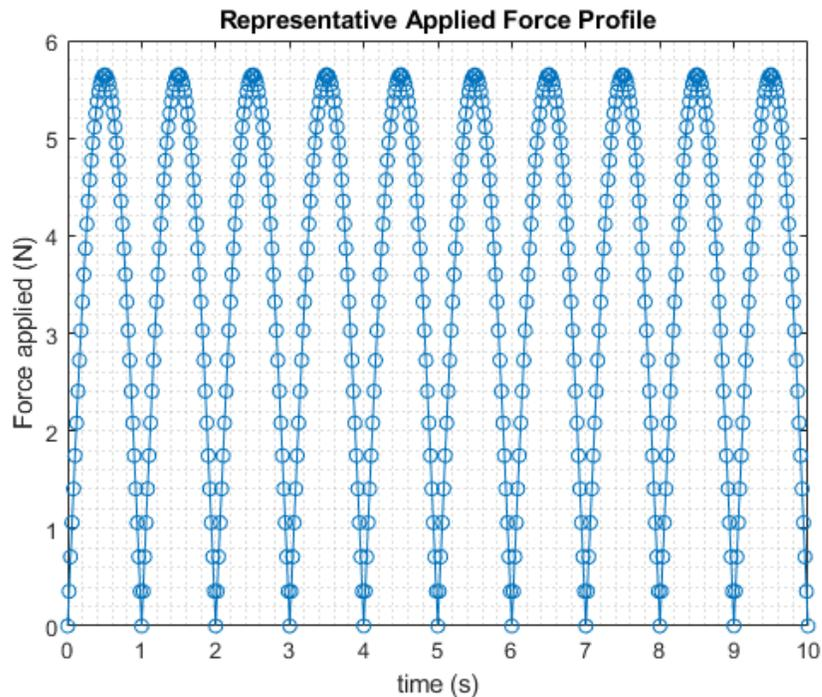
**Figure 9.** Ideal wave profile of a modulus sine wave.
