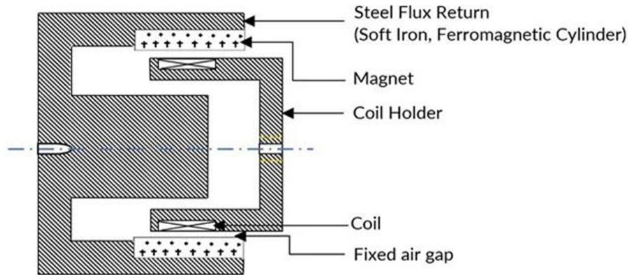
*Figure 5.* Diagram of a VCA with components labeled [8].
