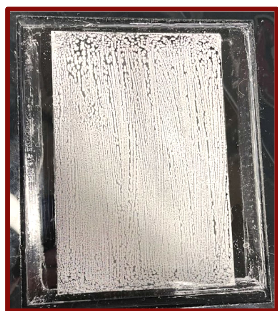
Figure 3. Example of Previous Team's Issue with Condensation
