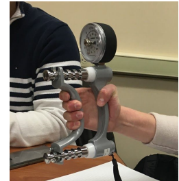
Figure 6: Demonstration of the JAMAR Hand Dynamometer
