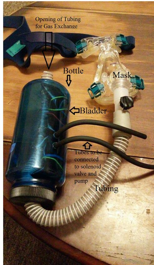
**Figure 1:** An image the final design built by last semester's design team. It features an inflatable bladder as the mechanism for varying dead space volume.
