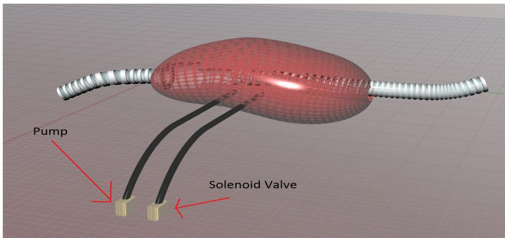
**Figure 2:** A CAD design of SBwP while apnea is detected (the body is inflated thus maximizing dead space). During normal breathing the body would be deflated and snug to the air tubes, thus minimizing dead space.
