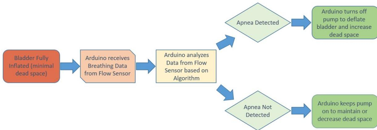
**Figure 4:** Flow Diagram of the function of the varying dead space system. The algorithm for detecting apnea will be utilized in the analysis of the voltage data from the flow sensor.
