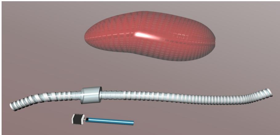
**Figure 3:** An image of SBwR with the parts separated for aid in visibility. When the design is fully assembled, the stepper motor/cover will be located in the air tube, and the air tube will be located in the soft body.
