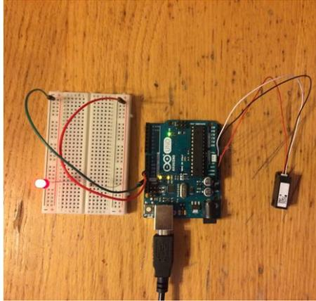
**Figure 5:** Apnea detection circuit including a flow sensor (right), microcontroller, and resistor LED combo (left). The LED lights up when an apnea is detected by the algorithm to show the circuit is working.
