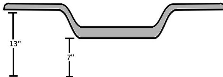
**Figure 3: Dip Bar-** Additional bending in the frame along the side of the device.
