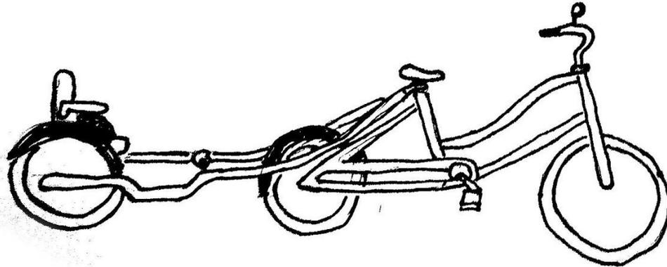
**Figure 5:** Final design consisting of a 2 wheeled, double framed trailer attachment. Contains independent drivetrain mechanism powering rear wheel of trailer.
