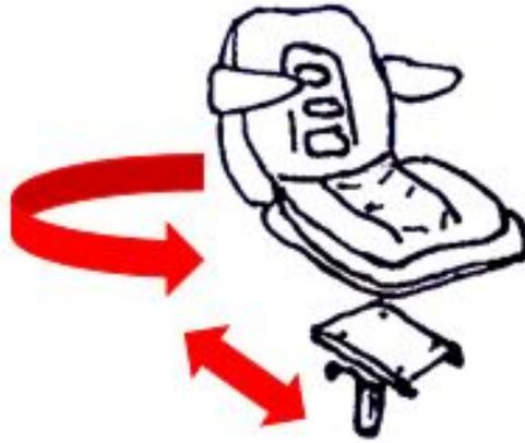
**Figure 1: Swivel chair-** The seat being used for our device will attach to a mechanism that would allow for a swivel action to occur.
