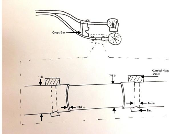
**Figure 2: Slide Bar-** An inner rod structure connected to the frame by removable screws along with additional cross bar for stability and strength.
