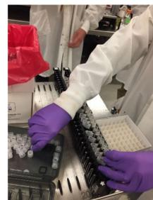
Figure 2: Technician manually uncapping sample tubes in the client's affiliated laboratory [2]
