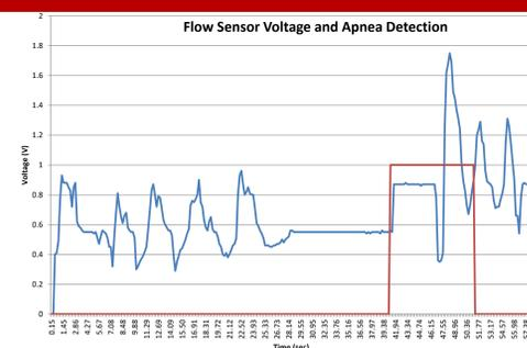
Figure 6. Flow sensor voltage and apnea detection data. The red line represents when apnea was detected and the blue line represents the breathing pattern of the test subject. Testing verified the functionality of the algorithm.
