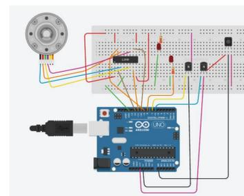
Figure 5. A schematic of the circuit that controls the stepper motor based on the readings from the flow sensor.
