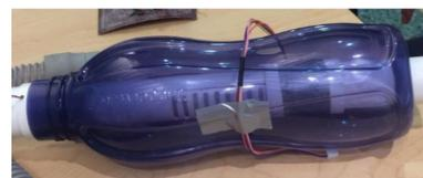
Figure 2. A hard waterbottle with PVC pipe through it was used as the body of the device. The PVC pipe has slits cut into it to vary dead space volume
