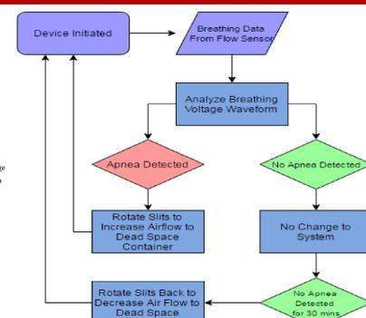
Figure 7. Apnea detection algorithm flow chart that drives the device as a dynamic and active apnea therapy system
