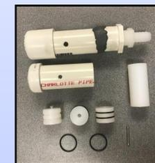
**Figure 5:** The above picture contains assembled and disassembled pieces of the shunt valve prototype.
