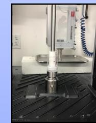
**Figure 6:** The prototype undergoing cyclic loading in the MTS machine.
