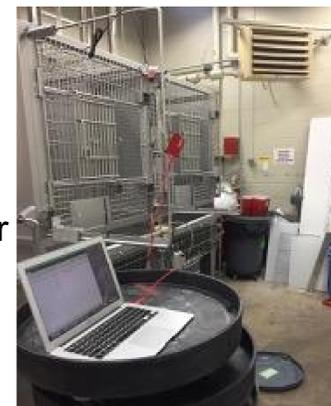
Figure 5: This image shows the setup of testing. Only one load cell was used on the top left corner.
