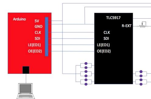
Figure 12. Block diagram of the circuit used in the LED excitation source. The TLC5917 is an 8-bit shift register.
