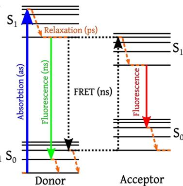
Figure 1. Diagram of FRET concept [2]
