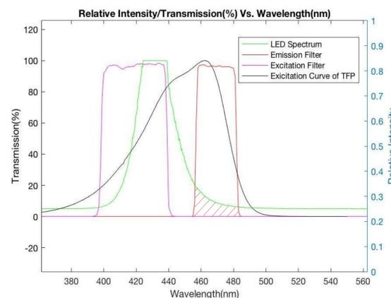
Figure 10. MATLAB analysis of optical components following testing
