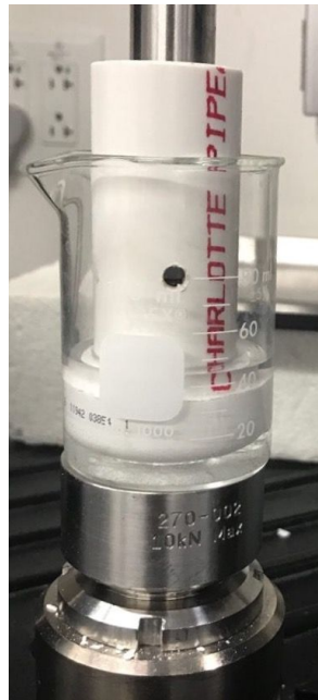
Figure 10. Example of set up for piston testing while the lower chamber was filled with water. Lubricated testing was performed similarly but the piston was lubricated with water and not immersed in water (by Andrew Miller).
