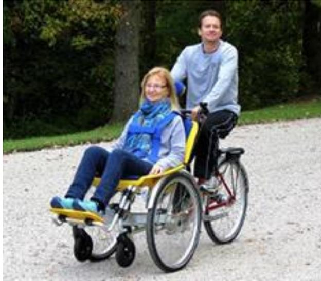
**Figure 2:** Competing design of a front end attachment tandem bicycle. This front end attachment is *The Duet* by Wheelchair Bicycle Tandem[7].
