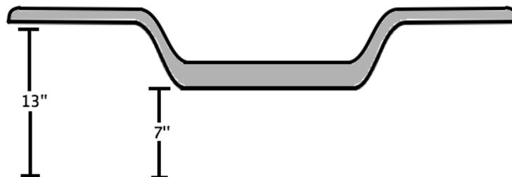
**Figure 6: Dip Bar-** Additional bending in the frame along the side of the device.
