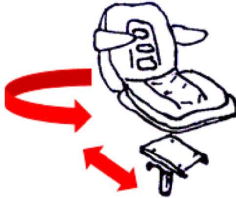
**Figure 4: Swivel chair-** The seat being used for our device will attach to a mechanism that would allow for a swivel action to occur as well as front and back movement.
