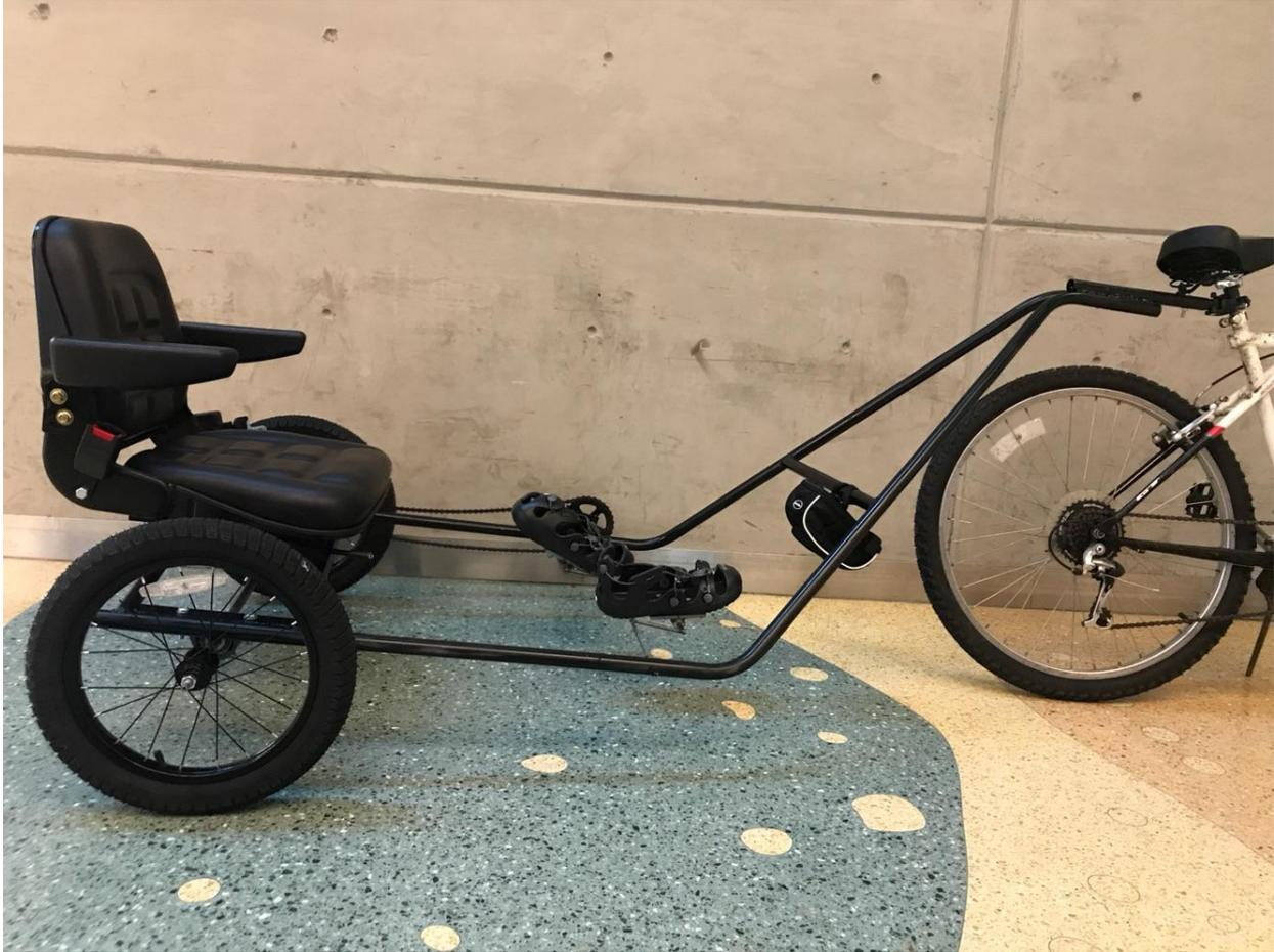
**Figure 7:** Final design consisting of a 2 wheeled, double framed trailer attachment. Contains independent drivetrain mechanism powering rear wheel of trailer.
