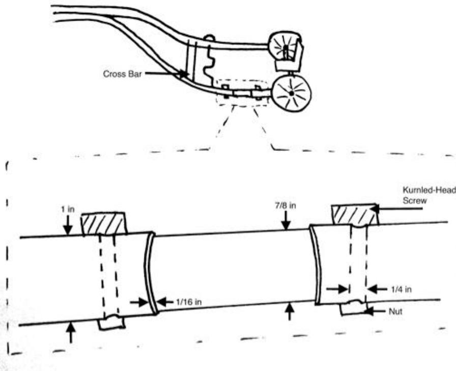
**Figure 5: Slide Bar-** An inner rod structure connected to the frame by removable screws along with additional cross bar for stability and strength.
