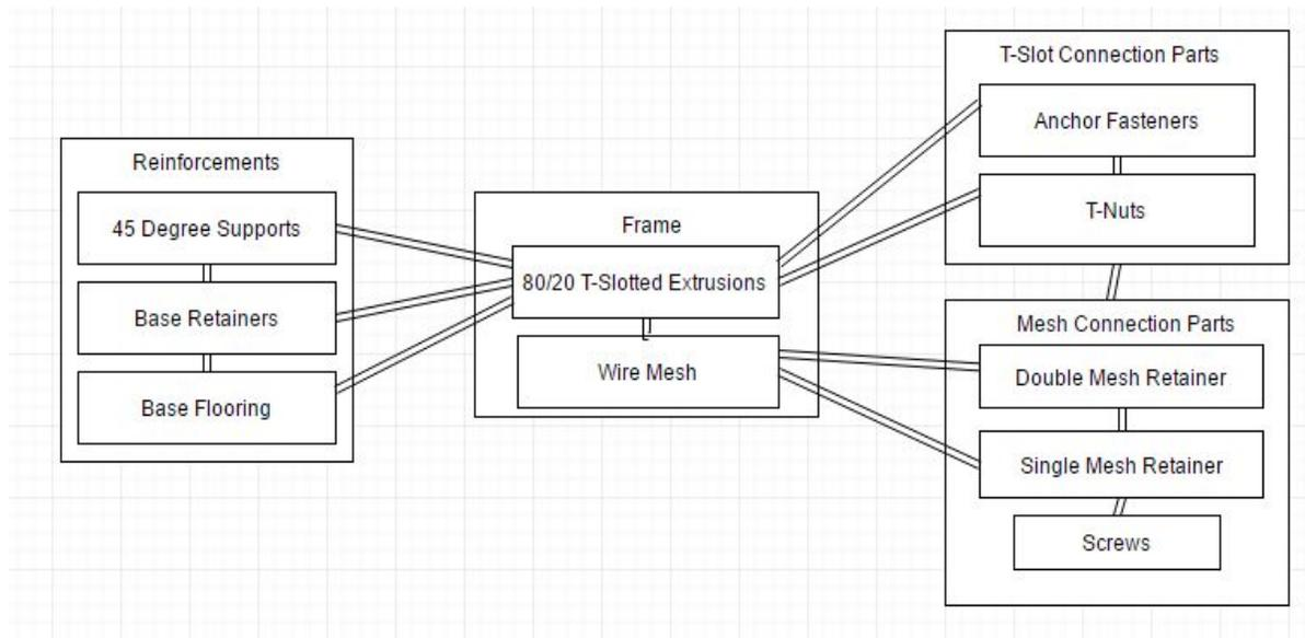
**Figure 1:** Product architecture for the Spider Cage design team. The connection clusters are fundamental to the assembly of the cage.
