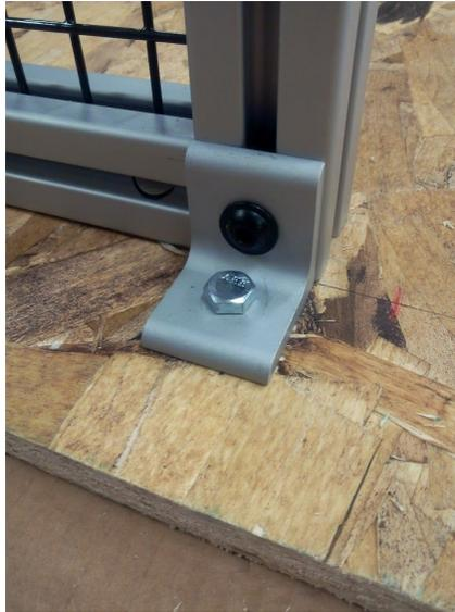
Figure 1: The front left corner bracket attached to the cage and the base flooring.
