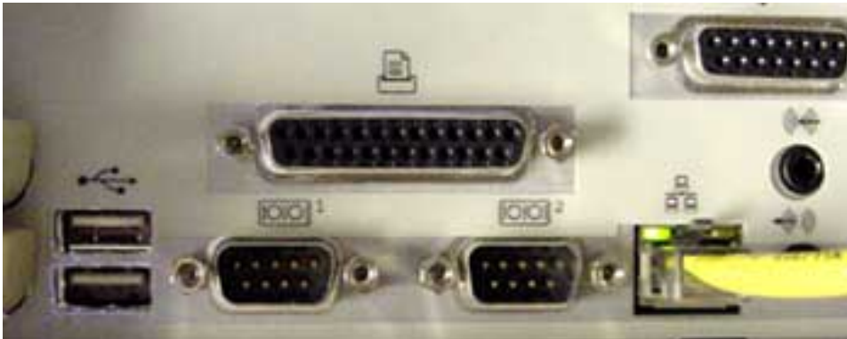
Figure 5. This figure above shows the serial port (we will be using the 2 smaller 9-bit ports on the bottom) (5)
