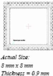
Figure 4: Picture and dimensions of surface mounted rechargeable battery
