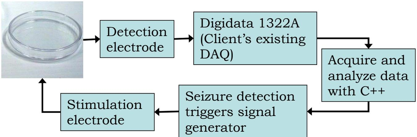
Figure 10: Schematic representation of our first design option
