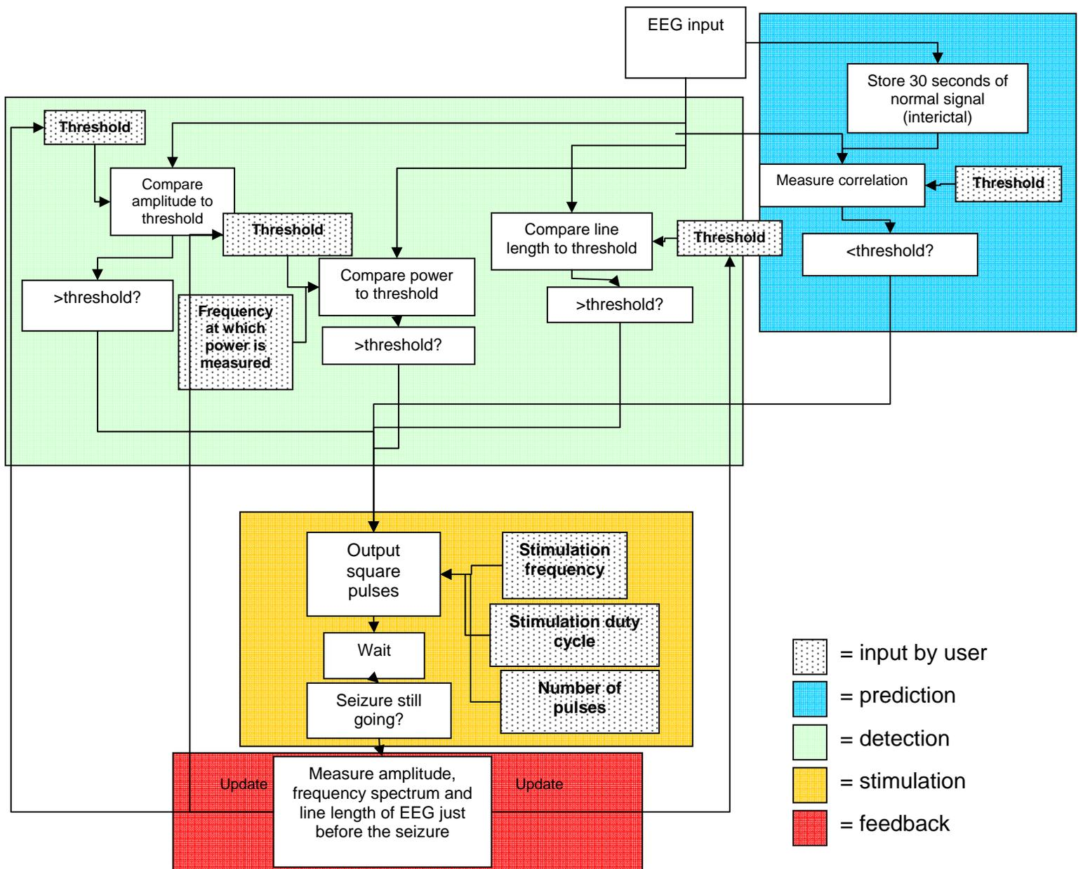
Figure 12: Simplified logical diagram for the functioning of our LabVIEW seizure detection algorithm
