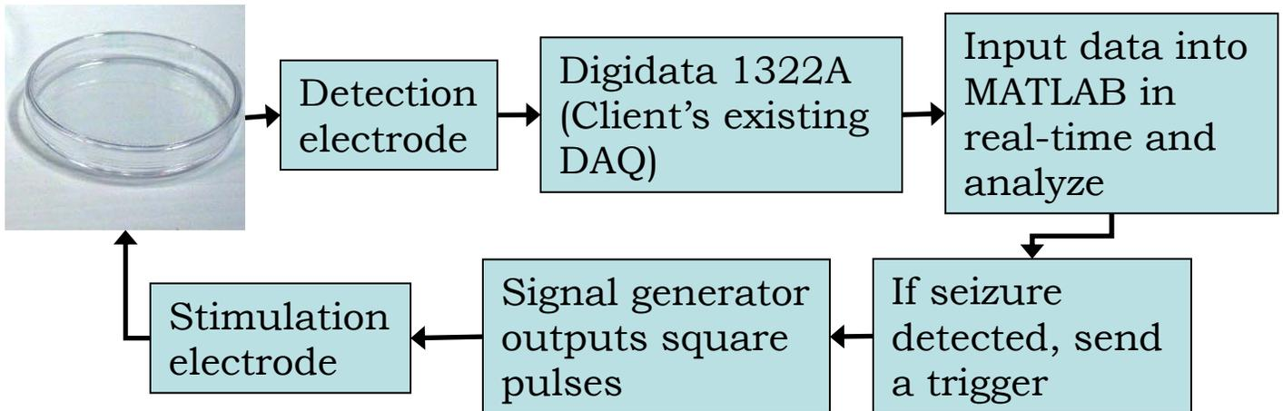
**Figure 11: Schematic representation of our second design option**
