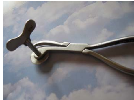
Figure 5 –Shown above is the device used to cut one side of the ring.
