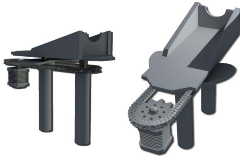
Figure 6. A computer generated image of the Belt Driven Rotator design, which rotates the experimental box, through a chain or belt, by a stepper motor which is placed outside of the electromagnetic field.
