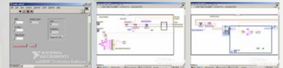
(Left) User interface to enter parameters. (Middle) Counter initialization. (Right) Breath control via communication with stepper motor.
