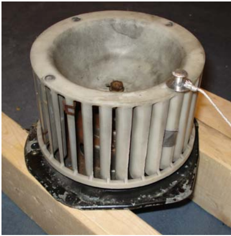
Figure 7: Fan Motor Bolt, washer, and string attached through outer rim of fan
