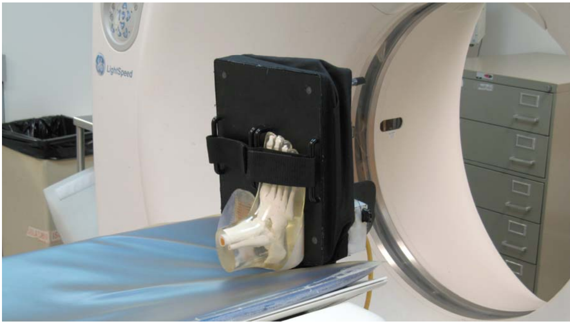
Figure 9 Photographs of the final prototype with a phantom foot in place, attached to the CT scanning table.
