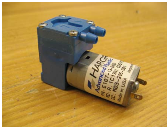
Figure 11 The diaphragm pump used to inflate the air bladder.
