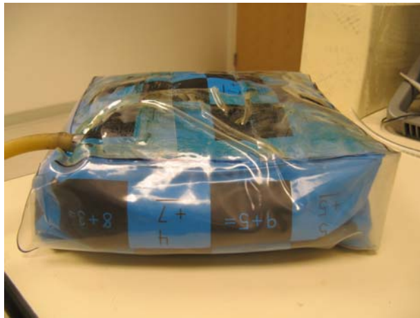
Figure 10 The air bladder with Polyfilm sheath to prevent bulging.
